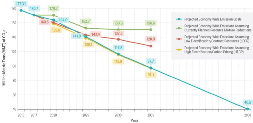
**Figure 1. New England Emission Reduction Goals Compared with Projected Reductions Due to: (1) Planned Renewable Resource Additions; (2) Such Additions with Increased Electrification; or (3) Such Additions with High Electrification and Carbon Pricing**
