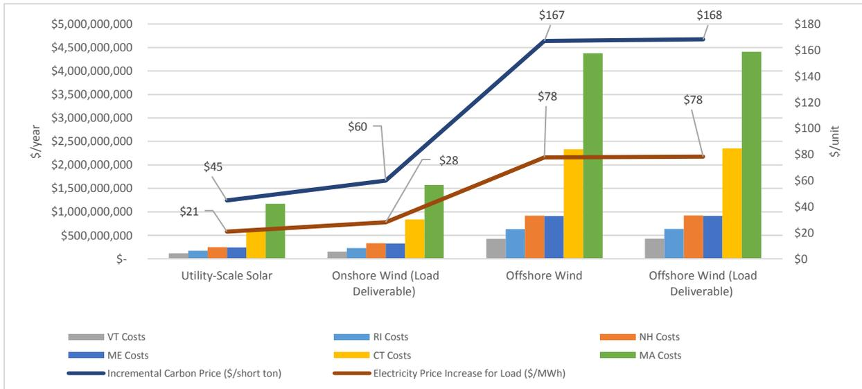
Figure 7 provides a breakdown of costs by state (based on the annual load ratio share and excluding pumping load and export transactions) as compared to the incremental carbon price and incremental energy price paid by load. These costs mirror the total payments made to suppliers, ranging from \$2.6-\$9.7 billion annually .
